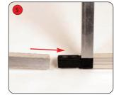
Push fit the bottom horizontal tubes into the 'A' frames, ensure the plastic joiners face inwards
