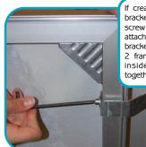
If creating inside corner, use wide angle bracket and place angle bracket around hex screw and under washer that is already attached to extrusion insert. Wide angle bracket will attach and go around outside of 2 frames connecting them to create an inside corner with 2 graphics coming together.
