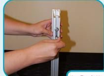
Use (3mm) Allen wrench to tighten set screw to set location of extrusion insert. Then, completely assemble frame and install graphics per SEG installation instructions.
