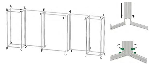
Step 3 - Top horizontal posts will have the same labels as the bottom horizontals with corner connectors attached. Slide top extrusion connectors down onto tops of vertical posts. Tighten D screws on vertical posts.
