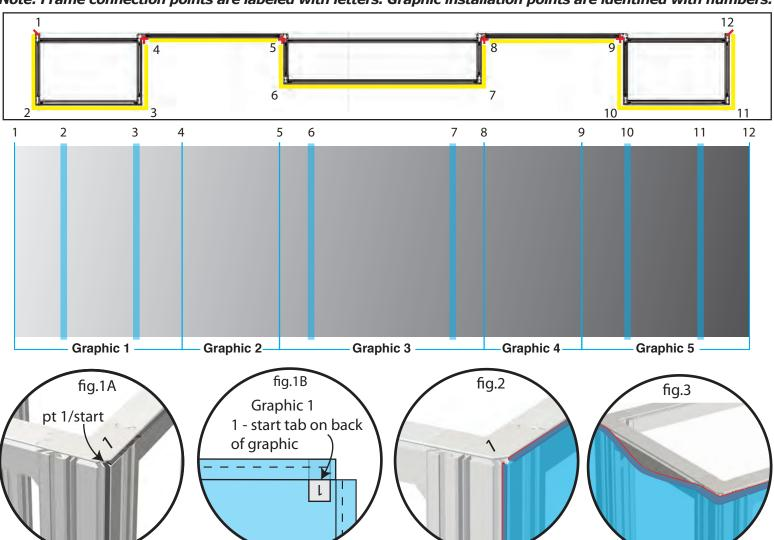
Step 1 - Identify start point on top of frame (fig. 1A, label-1) and Step 2 - Insert 1 Top corner of graphic top left corner with start tab (fig. 1B, shown in blue).
