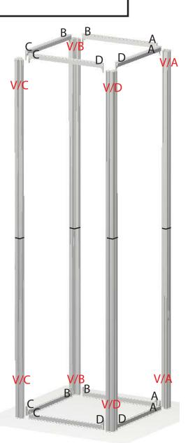
Step 3 - Place assembled vertical posts down onto corner connector on horizontal section.
