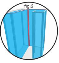
Step 6 - Insert welt in vertical grooves between top and bottom corners.
