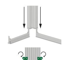
Step 3 - Top horizontal posts will have the same labels as the bottom horizontals with corner connectors attached. Slide top extrusion connectors down onto tops of vertical posts. Tighten D screws on vertical posts.
