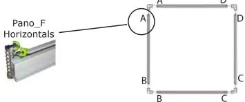
Step 2 - Assemble vertical posts. 4 long and 4 short lengths. Vertical extrusions are labeled with the letter that corresponds to the adjoining horizontal piece. The
