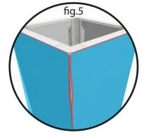
Step 5 - Insert welt in vertical grooves between top and bottom corners.
