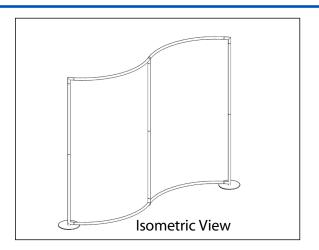
2) Base plates connect into threaded end posts of frame.
