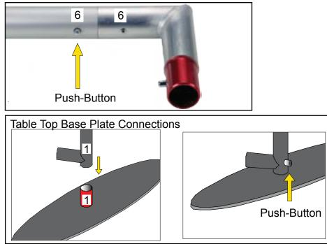
Base Plate Connections are made by holding the button down and sliding the red tube into the opposing tube on base until it locks in place.
