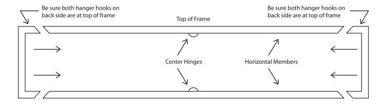
Make sure all pieces are fully pushed together. Align magnets on end of header with magnets at end of frame. Roll the header onto the frame, line up magnets and gently push into place. Place complete header and header frame on top of display with extended hooks going over top of display. Be sure the hooks are on top of the pop-up frame. The display panels (ie, the walls) will not support the header.
